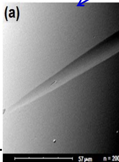
Scratch Test Microtest MTR2
