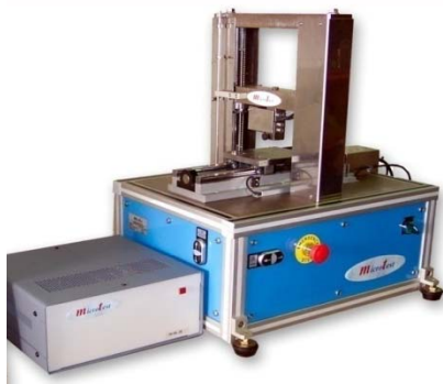
Scratch Test Microtest MTR2
