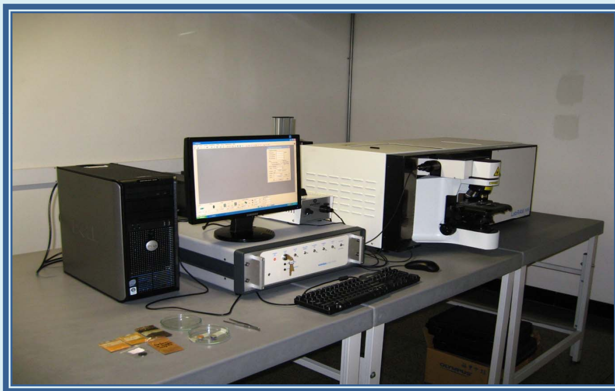
MICRO-RAMAN Jobin Yvon, Model Labram HR
